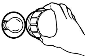
3. Turn bulb counterclockwise to remove from socket.
