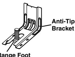
**To verify the anti-tip bracket is installed and engaged:**
