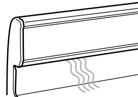
The oven vent releases hot air and moisture from the oven, and should not be blocked or covered. Blocking or covering the oven vent will cause poor air circulation, affecting cooking and cleaning results. Do not set plastics, paper or other items that could melt or burn near the oven vent.
