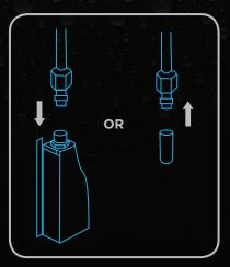
If you don't have an ice maker, skip this step. Simply leave the cap on the dispenser's refrigerator line and move on to step 9.
