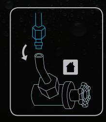
Disconnect the water line that is running between your refrigerator and the house at the refrigerator end.
