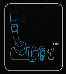
Turn your house's water back on. Make sure water isn't leaking anywhere. If it is, check the connections and tighten if necessary.
