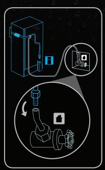
Disconnect the old hose from your house water line and replace it with the dispenser's house water line. Use your hand to tighten the nut, then use a wrench to give it a half-turn.
