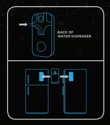
Route the dispenser's tubing through the prongs on the back of the unit and place the dispenser on the front or side of your refrigerator with its integrated magnets. If hanging on the front, mount the dispenser 2–3 inches from the hinge side to allow the tubing to move freely within the Tubing Holders on the side.
