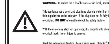
WARNING - To reduce the risk of fire or electric shock, DO NOT do not use this fan with a solid-state speed control device.
