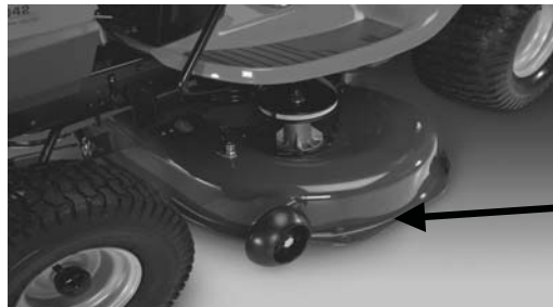
Stamped Deck Shell below, NOT reinforced
