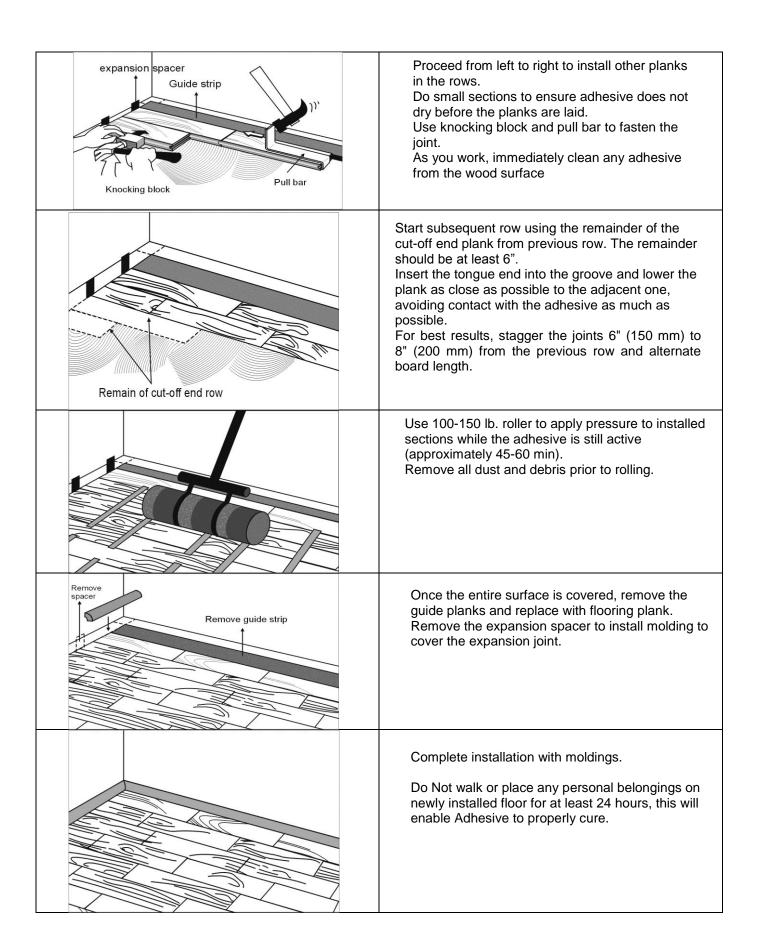
IMPORTANT: During Installation, immediately wipe any adhesive from the floor surface using Bostik's Ultimate solvent and/or wipes.
