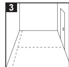
3. Measure and mark centerline. Centerline must be square to line as in step 1.
