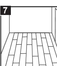
7. Install all full planks (A) before making a perimeter cuts. Helpful hint: You can step on the planks (A) immediately after installation, or sit on the floor during the installation.
