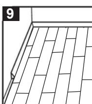
9. Roll installed floor with a 100 lb. roller (not included) prior to installing optional quarter round-molding (not included) to finish job.
