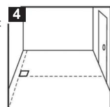
4. Remove release paper from a plank (A) to expose adhesive. Lay the first plank (A) in the corner of the first line and the centerline. Caution: Discard the release paper immediately after removing it from all planks (A).
