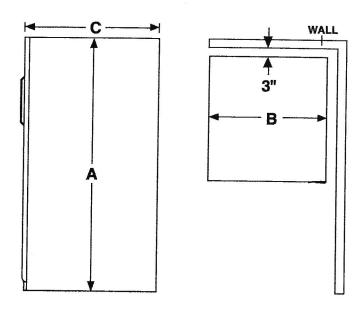
Allow sufficient clearance on hinge side of freezer when installing next to a wall where handle may make contact.
