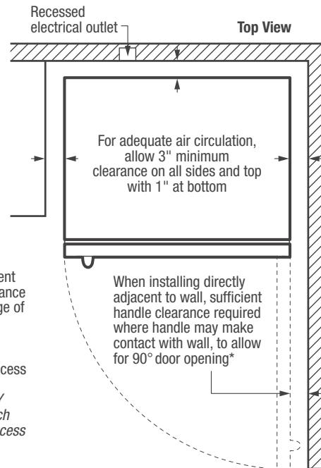
\* When installing freezer adjacent to wall, cabinet or other appliance that extends beyond front edge of unit, 20" minimum clearance recommended to allow for optimum 140° door swing, providing complete basket access and removal. (Absolute 3" minimum clearance will ONLY allow for 90° door swing which will provide limited basket access with restricted removal.)
