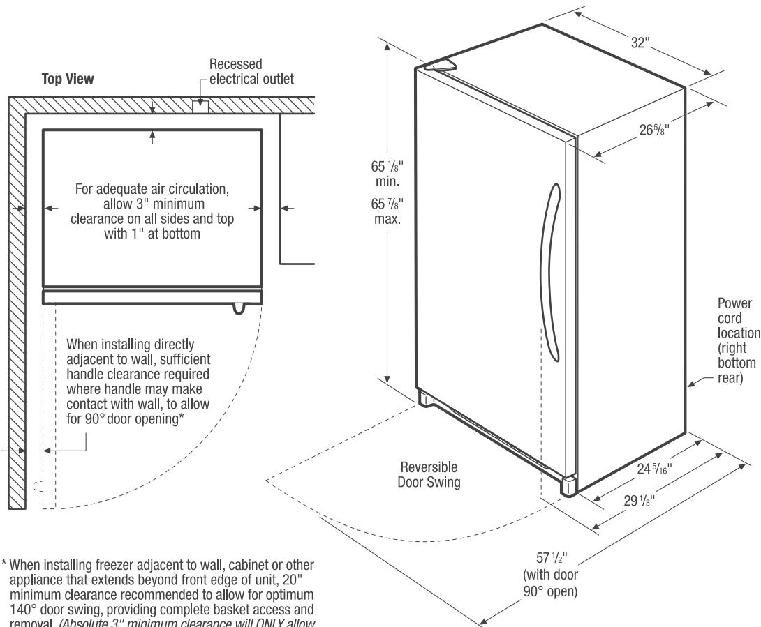
\* When installing freezer adjacent to wall, cabinet or other appliance that extends beyond front edge of unit, 20" minimum clearance recommended to allow for optimum 140° door swing, providing complete basket access and removal. (Absolute 3" minimum clearance will ONLY allow for 90° door swing which will provide limited basket access with restricted removal.)
