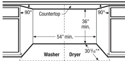
**Side-by-Side Units in Under-Counter Installation**
