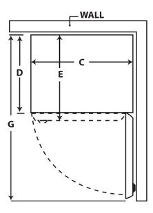
Allow sufficient clearance on hinge side of refrigerator when installing next to a wall where handle may make contact.
