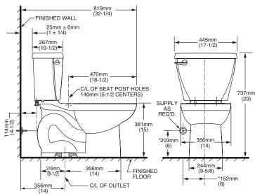
THIS TOILET IS DESIGNED TO ROUGH-IN AT A MINIMUM DIMENSION OF 356MM (14") FROM FINISHED WALL TO C/L OF OUTLET. SUPPLY NOT INCLUDED WITH FIXTURE AND MUST BE ORDERED
