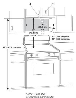
**NOTE:** The grounded 3 prong outlet must be inside the upper cabinet.
