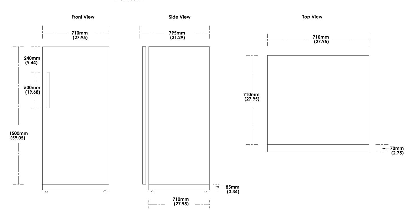
\*Air Circulation Clearance: \*Side: 2" (50mm) \*Top: 2" (50mm) Back: 2" (50mm)
