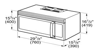
Measurements in inches (mm) in brackets
