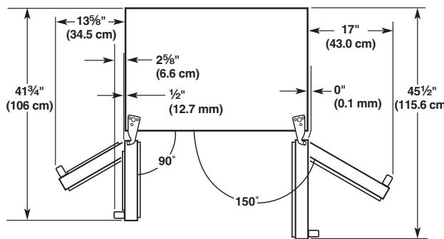
Location must permit doors to open to a minimum of 150°. Allow 13-1/4" (34 cm) minimum space between the side wall and the freezer side of the refrigerator. Allow 16-1/2" (42 cm) minimum space between the side wall and the refrigerator side.
