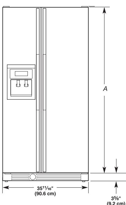
■ Height dimensions are shown with the leveling legs extended to the minimum height of 1/4" (6.4 mm) below the refrigerator.
