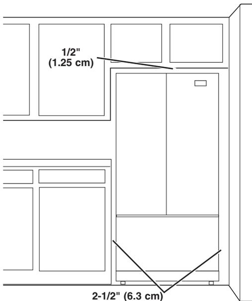
To ensure proper ventilation for your refrigerator, allow for 1/2" (1.25 cm) space at the top and behind the refrigerator. When installing your refrigerator next to a fixed wall, leave 2-1/2" (6.3 cm) minimum on both sides to allow for the doors to swing open. If your refrigerator has an ice maker, allow extra space at the back for the water line connections.
