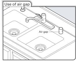
Make sure to use an air gap if the drain hose is connected to house plumbing lower than 20" (50.8 cm) above subfloor or floor.
