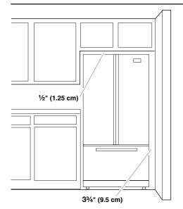
To ensure proper ventilation for your refrigerator, allow for a  $\frac{1}{2}$ " (1.25 cm) space at the top and behind the refrigerator. If your refrigerator has an ice maker, allow extra space at the back for the water line connections. When installing your refrigerator next to a fixed wall, leave 3<sup>3</sup>/<sub>4</sub>" (9.5 cm) minimum space between the refrigerator and wall to allow the door to swing open.
