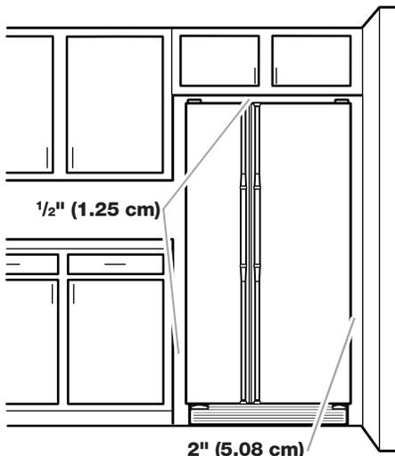
To ensure proper ventilation for your refrigerator, allow for ½" (1.25 cm) of space on each side and at the top. Allow for 1" (2.54 cm) of space behind the refrigerator. If your refrigerator has an ice maker, allow extra space at the back for the water line connections. When installing your refrigerator next to a fixed wall, leave a 2" (5.08 cm) minimum space on each side (depending on your model) to allow the doors to swing open.
