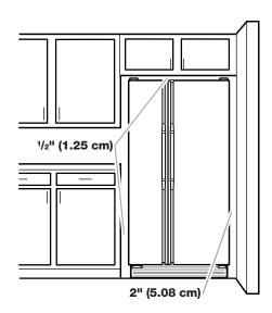
To ensure proper ventilation for your refrigerator, allow for  $\frac{1}{2}$ " (1.25 cm) of space on each side and at the top. Allow for 2" (5.08 cm) of space behind the refrigerator. If your refrigerator has an ice maker, allow extra space at the back for the water line connections. When installing your refrigerator next to a fixed wall, leave a 2" (5.08 cm) minimum space on each side (depending on your model) to allow the doors to swing open.
