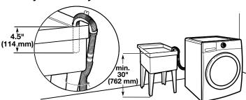
Minimum capacity: 20 gal. (76 L). Top of laundry tub must be at least 30" (762 mm) above floor; install no higher than 96" (2.44 m) from bottom of washer.
