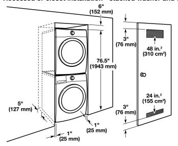
All dimensions show recommended spacing allowed, except for closet door ventilation openings which are the minimum required.
