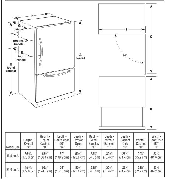
To ensure proper ventilation for your refrigerator, allow for a  $\frac{1}{2}$ " (1.25 cm) space on each side and at the top. Allow at least 1" (2.54 cm) between back of cabinet and the wall. If your refrigerator has an ice maker, make sure you leave some extra space at the back for the water line connections.
