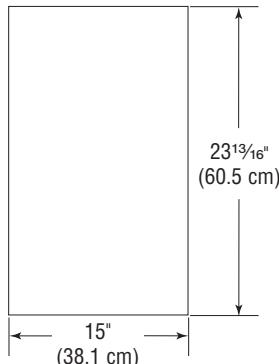
Panel should be  $\frac{1}{2}$ " to  $\frac{5}{8}$ " (13 to 16 mm) thick.
