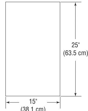
Panel should be  $\frac{1}{2}$ " (13 mm) min. thickness.
