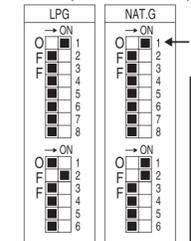
Move switch 1 to OFF for long flue lengths. See below.
