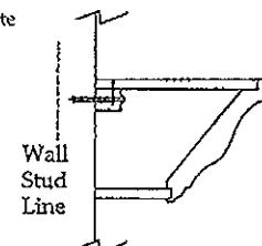
Fig. 2 Cross-sectional view of shelf, wall, and cleat assembly
