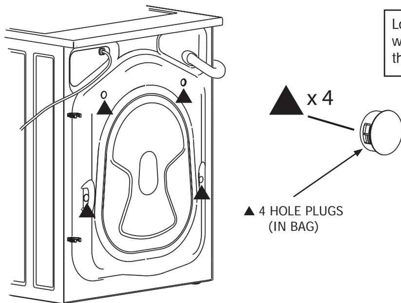
Locate 4 hole plugs in the small bag supplied with washer instruction guides. Insert them in the holes in washer back panel.
