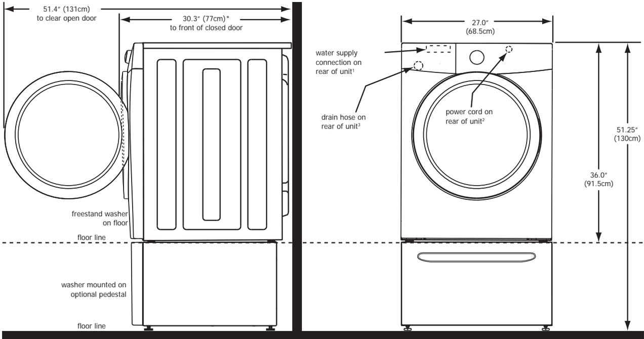
\* To obtain these minimal depth dimensions, dryer must be vented straight back. Using a quick-turn 90° elbow (right or down on freestanding dryer) adds approximately 0.75 in. (2.0 cm) to installation depth. Upward venting of exhaust on pedestal-mounted or freestanding dryer adds approximately 4 in. (10.2 cm) to installation depth. Leftward venting on pedestal-mounted or freestanding dryer adds approximately 3.75 in. (9.5 cm) to installation depth.
