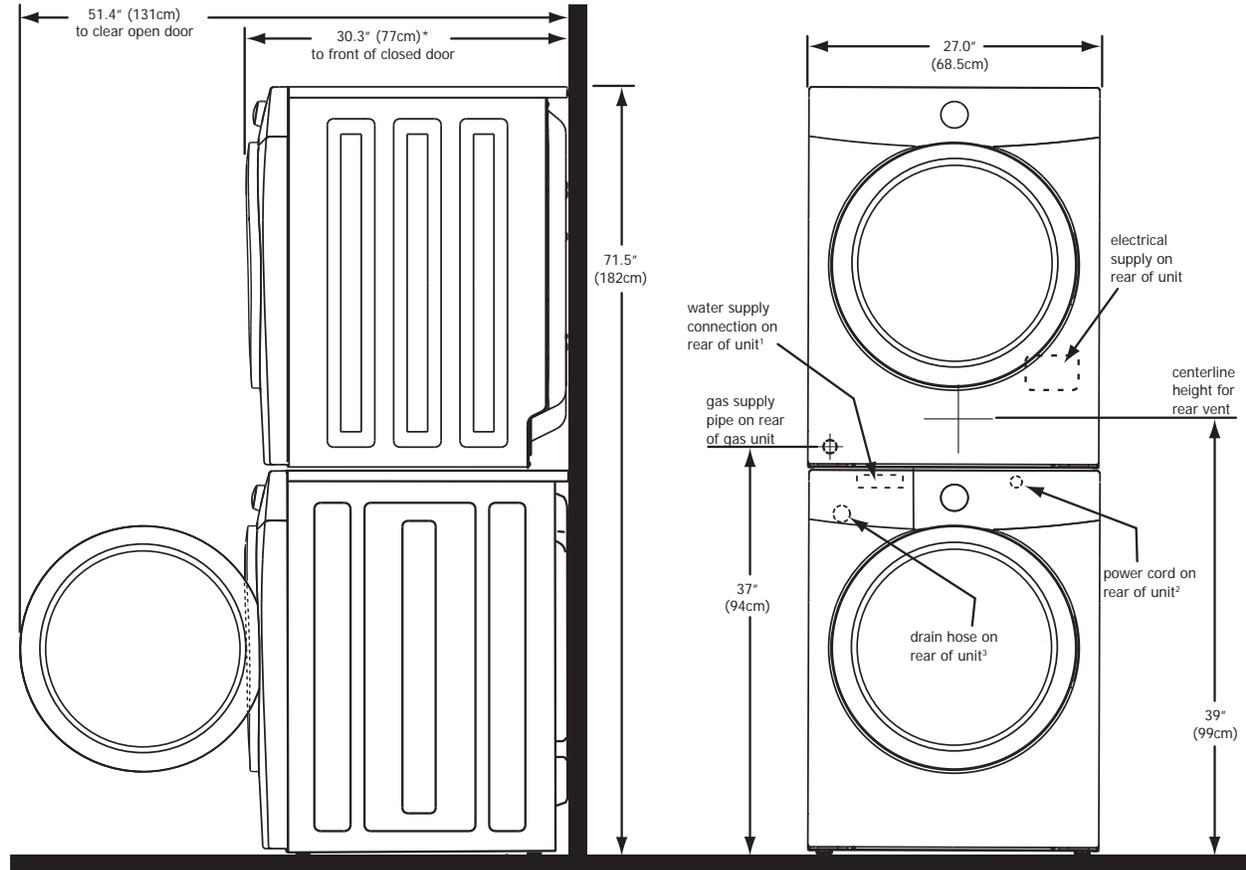
\* To obtain these minimal depth dimensions, dryer must be vented straight back. Using a quick-turn 90° elbow (right) adds approximately 0.75 in. (2 cm) to installation depth. Upward venting of exhaust on stacked dryer adds approximately 4 in. (10.2 cm) to installation depth. Downward venting of exhaust on stacked dryer adds approximately 2.25 in. (6.5 cm) to installation depth. Leftward venting of exhaust on stacked dryer adds approximately 3.75 in. (9.5 cm) to installation depth.
