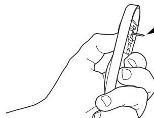
**CAUTION:** Pin is sharp and should be handled with care. Always be sure drywall pin is closed when not in use.
