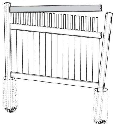
For open top picket fences follow Step 11 for assembly. Attach middle rail into left side of post route only then guide rail over boards. Insert top rail into left post route holes of first post only.
