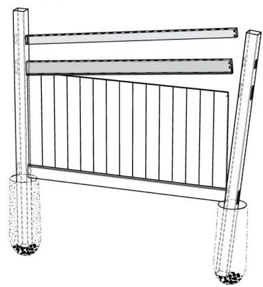
Insert pickets down through top and middle rail. Note: Scalloped and Arched panels have pickets/boards that are numbered. Start from left side with the #1 picket/board first.
