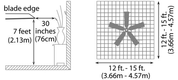
This fan can be mounted *only* as a **flushmount** on a regular ceiling. **Downrod** installations are **not** available for this fan.
