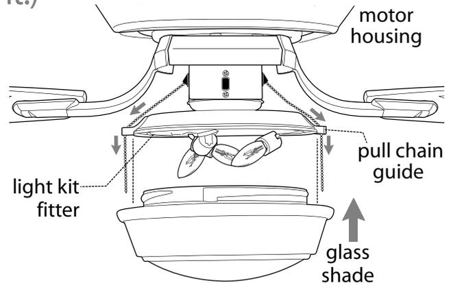
**If you wish to use fan WITHOUT the light kit,** remove hex nut and lock washer from threaded rod at top of light kit fitter. Remove switch housing cap. Locate small plastic cap in hardware pack and insert cap firmly into hole in middle of switch housing cap.
