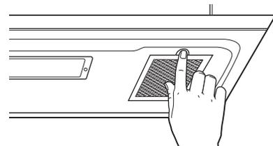
**6** Install grease filters. See the Owner's Manual packed with the oven.
