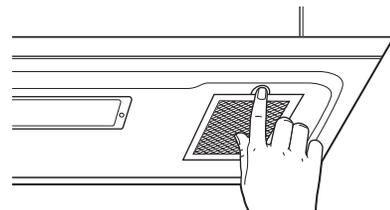
**7** Install grease filters. See the Owner's Manual packed with the oven.
