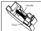
**IMPORTANT:** Improper alignment or positioning of the water tank will cause the unit to pause operation, the warning light on top of the dehumidifier will illuminate followed by a beeping sound, until the water tank is fitted properly.
