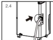
**IMPORTANT:** Make sure water can flow down the garden hose by keeping the hose angled down and free of bends or kinks.
