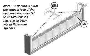
B. Place a "FLAT" spacer on top of the first and last block of the previous row where they meet the side channels. C. Set the first block and last block of the next row into the side channels on top of the "FLAT" spacers.
