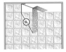
M. Screw the short leg of the anchor to the top of the opening.
