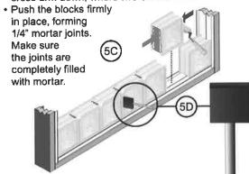
D. Remove excess mortar with a polyfoam brush, and fill any voids on both sides of the panel.
