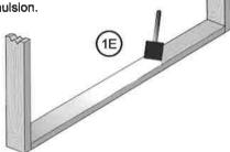
If using Weldbond®, apply mortar to the surface before it cures. Otherwise, let the treated area set up and cure before installing the first row of block.
