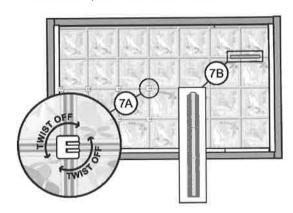
B. With moderate pressure, run the striking tool over all the joints. It is best to strike all the horizontal joints first, then the vertical joints so the pattern is uniform. Fill any voids with mortar.
