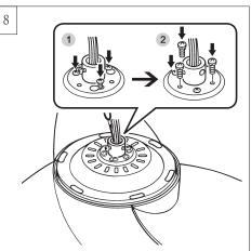
Replace the top plate removed in step 5, aligning holes by turning the plate clockwise till lock, and then reinstall the screws removed in step 5. Tighten all screws securely.
