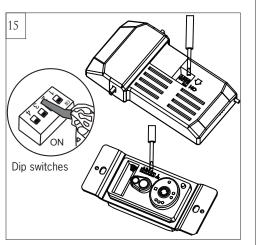
Set dip switches on the Remote Transmitter and Remote Receiver to the same settings. This must be done so the units will communicate properly. If you have other fans you can set to control from one Transmitter by setting receivers the same as the Transmitter. If you have more than one fan with remote, you can set the dip switches to different positions to have separate control
