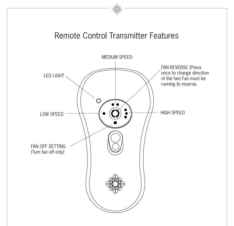
FAN SPEED: Depress "1 dot" for low speed, "2 dots" for medium or "3 dots" for high. To turn fan off press square".
