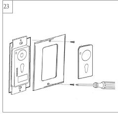
Attach front cover to wall control unit with screws provided. Snap battery cover in place
