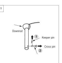
Remove preassembled keeper pin and cross pin from downrod.
