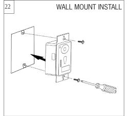
Install wall control unit to outlet box using machine screws provided.
