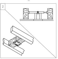
Before installing this fan make sure the outlet box is properly installed to the house structure. To reduce the risk of fire, electric shock, or personal injury, mount to outlet box or supporting system acceptable for fan support. (Mounting must support at least 35 lbs.) Mounting bracket
