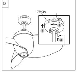
Lift canopy up, aligning its keyhole slot with the preassembled screw on mounting bracket and twist counterclockwise to lock in place. Reinstall the screw removed in step 17 and tighten all screws securely.
