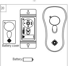
Remove battery cover. Install 12V battery into wall remote. Duracell MN21 / Evereday A23 / GP 23A all 12V. Attach cover of remote by placing over buttons and snap the battery cover in place.
