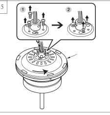
Remove every other screws located at round holes areas as shown in inset marked 1, keep screws. Partially loosen the other set screws located at keyhole slots as shown in inset marked 2. Remove the top plate by turning counterclockwise and take it up.
