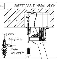
For Canadian installation and for USA fan and light kit combinations over 35 lbs, in both flush and downrod modes the safety cable must be installed into the house structure beams using 3" lag screws, washers and lock washers provided. Make sure that when the safety cable is fully extended the lead wires are longer than the cable and no stress is placed on the lead wires.
