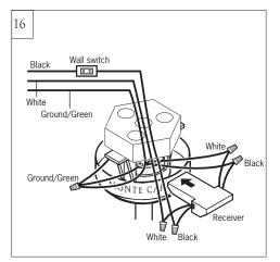
Make wiring connections using wire connectors provided as indicated above. White from fan to White from remote marked N. Black from fan to Black from remote marked L. White from house to White from remote marked AC N. Black from house to Black from remote marked AC L. Connect all green grounded wires to Grounded wire from House. Make sure that no filaments are outside of the wire connectors.
