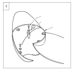
Put blades together, aligning the holes each other and then assemble the blades with wood set screws and washers provided.
