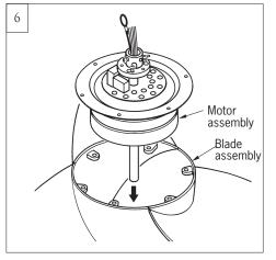
Place motor assembly onto blade assembly, aligning the holes on the plate of motor assembly with the screw holes on the blades.
