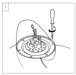
Install the motor assembly with the blade assembly using the screws provided. Tighten all screws securely.
