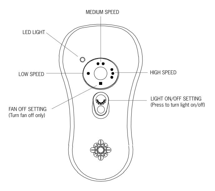
**FAN SPEED**: Depress "1 dot" for low speed, "2 dots" for medium or "3 dots" for high. To turn fan off press square".
