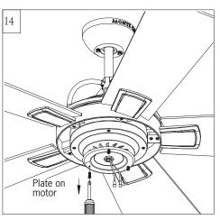
Loosen 2 and remove 1 preassembled set screws from the plate on motor. Save screw for later use.
