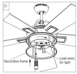
Attach decorative frame onto the plate on motor, threading the lead wires from fan through the decorative frame and aligning the keyhole slots on decorative frame with the preassembled screws on the plate. Twist clockwise till lock. Reinstall the screw removed in step 14. Tighten all screws securely.
