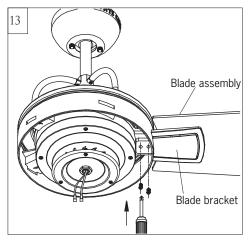
Insert blade assembly into the slot on flywheel.
