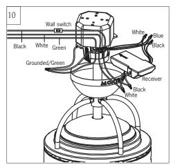
Make wire connections using wire connectors provided as indicated above. White from fan to White from remote marked N. Blue from fan to Blue from remote marked light. Black from fan to Black from remote marked L. White from house to White from remote marked AC N. Black from house to Black from remote marked AC L. Connect all green grounded wires to Grounded wire from House. Make sure that no filaments are outside of the wire nuts.
