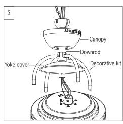
Place downrod over canopy, decorative kit and yoke cover. Thread lead wires and safety cable from motor assembly through downrod.
