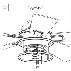
Attach light fixture onto the plate on the decorative frame, aligning the keyhole slots on the light fixture with the screws on the plate and twist clockwise till tight. Reinstall the screw removed in step 16. Tighten all screws securely.
