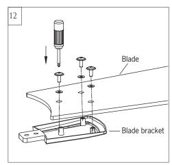
Install blade bracket with blade by 3 blade screws and washers provided. Tighten securely. Repeat this process for remaining blades.
