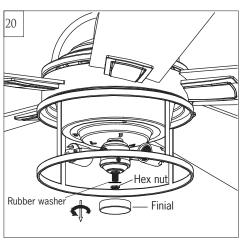
Remove rubber washer, hex nut and finial from light fixture. Save parts.
