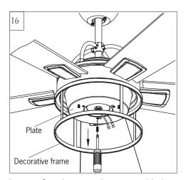
Loosen 2 and remove 1 preassembled screw from the plate on decorative frame. Save screw for later use.
