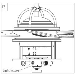
Connect white wire from fan to white wire from light fixture and then connect blue wire from fan to black wire from light fixture.
