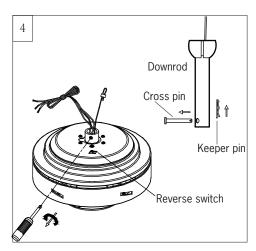
Partially loosen downrod set screws from yoke at top of motor assembly. Remove preassembled Keeper pin and cross pin from downrod.
