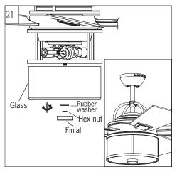
Attach glass onto light fixture. Install the rubber washer, hex nut and finial removed in step 20 to the thread rod by screwing to secure the glass. Do not over tighten the hex nut and finial.
