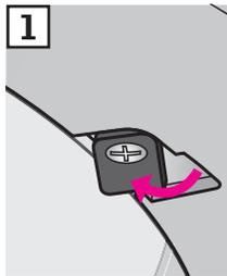
**ENGLISH:** Install the diffuser with the frosted side facing down. Secure the diffuser by rotating the plastic locks into locked position **1**.
