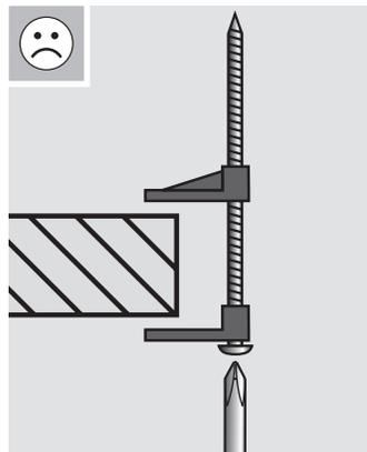
**ENGLISH:** Tip the plastic pins down into hidden position **A**. Insert the ceiling ring. Avoid distortion of the ceiling ring causing the diffuser not to fit smoothly **B**.
