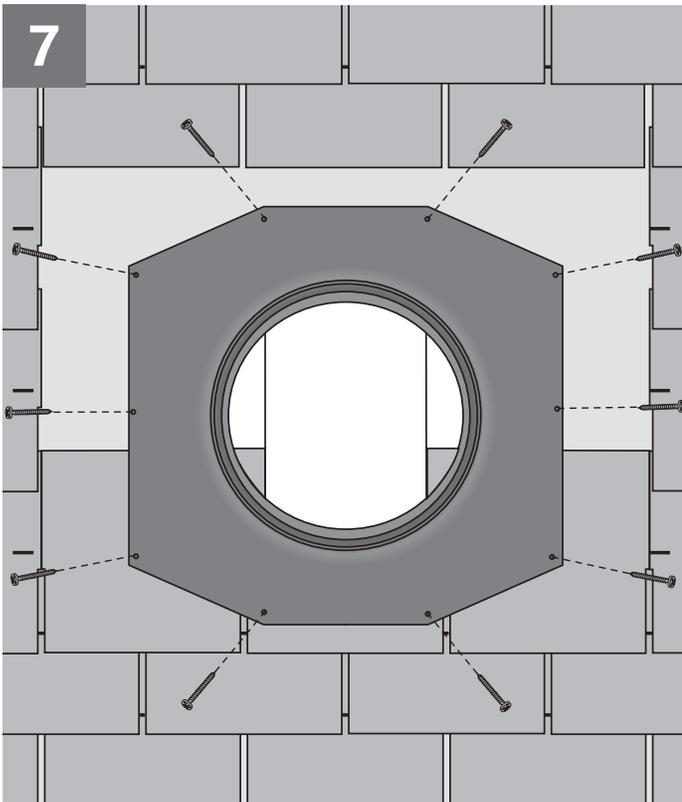
**ENGLISH:** Center the flashing over the rough opening and secure the flange with ten of the provided 1½" (40 mm) screws in all the pre-punched holes along the edges.
