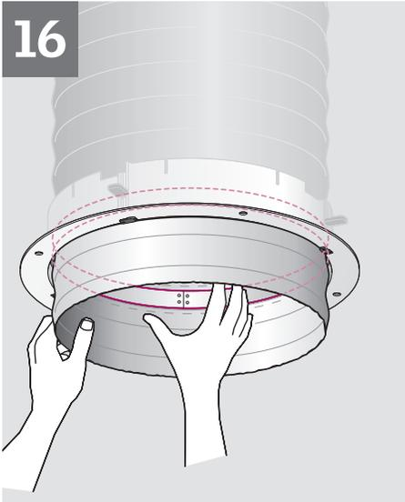
**ENGLISH:** Move the locking snap ring to final position as shown –  $\frac{3}{8}$ " (10 mm) above the position for the diffuser.
