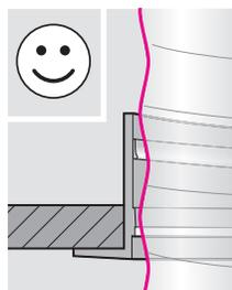
**ENGLISH:** Fold and insert the 1" (25 mm) locking snap ring to lock the flexible tunnel in place. Pull the flexible tunnel tight.
