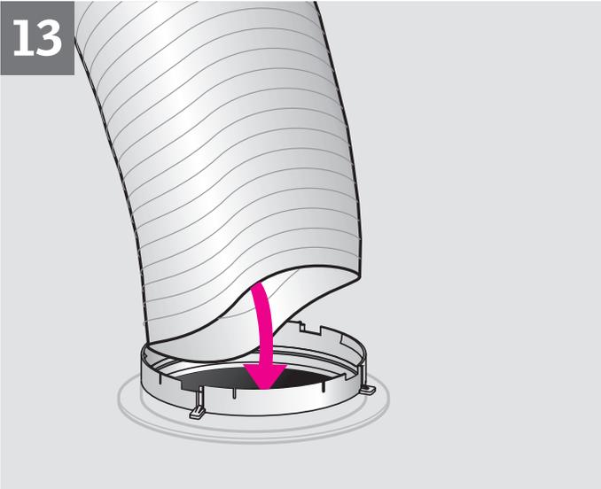
**ENGLISH:** Pull the flexible tunnel section down through the ceiling ring.
