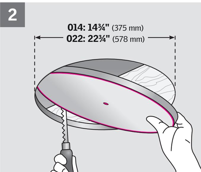
**ENGLISH:** From the inside, locate the nail indicating the center of the sun tunnel in the ceiling, mark circle and cut rough opening in the ceiling as shown.
