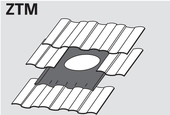
**ENGLISH:** Sun tunnel tile roofing – Refer to tile kit ZTM for installation in tile roofing.
