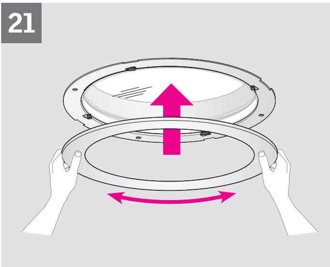
**ENGLISH:** Install the trim ring by aligning notches and rotate to secure.
