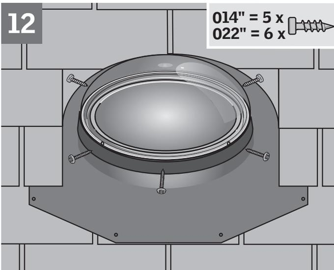
**ENGLISH:** Align holes; install and secure the dome with the 3/4" (19 mm) screws provided. Do not overtighten the screws.
