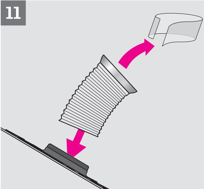
**ENGLISH:** Insert tunnel assembly into the flashing and seat the pivot ring into the intermediate ring. Secure with screws, if needed. Remove protective film.
