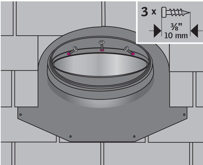
**ENGLISH:** Secure the pivot ring with screws if needed.
