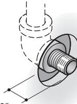
The nipple should extend 7/16" (1.1 cm) past the finished wall.
