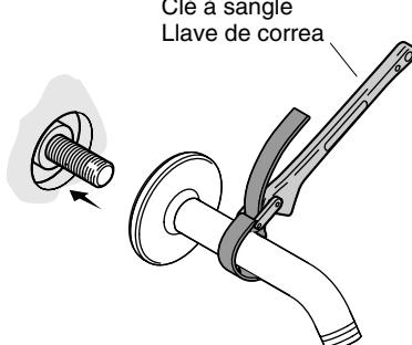
**11** Apply sealant tape. Install the showerhead.
