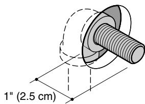
The nipple should extend 1" (2.5 cm) past the finished wall.
