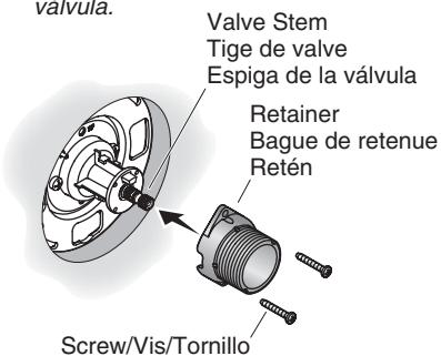
**b** Place the spacer and retainer on the valve stem. Secure with two screws.
