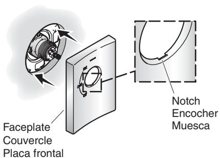
**23** Install the pivot ring to the faceplate and rotate clockwise to lock in place.
