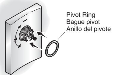
**24** Turn the valve stem counterclockwise to the "OFF" position.
