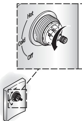
**25** Position the stem adapter on the valve stem. Secure with the screw. Position the handle on the stem adapter with the handle down. Hold the handle and turn the bonnet to thread it into the valve.
