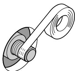
**10** Carefully tighten the shower arm using the strap wrench.
