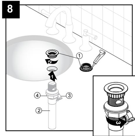
Apply silicone to the underside of the flange (1). Insert the pop-up body (2) into the sink. Screw the flange (1) onto the pop-up body (2). The pivot hole (3) must face the back of the sink. Use the groove joint pliers to tighten the nut (4), but do not over tighten. Do not turn the pop-up body (2) while tightening the nut (4) or the sealant may not seal properly. Clean away any excess sealant.
