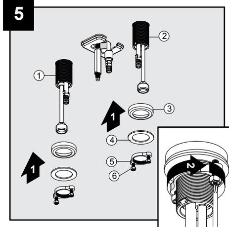
Secure the end valves (1 & 2) with the mounting brackets (3), washers (4) and the nuts (5). Hand tighten the nuts (5) onto the end valve (1 & 2) shanks. Lock the nuts (5) into position by tightening the screws (6) with a Phillips screwdriver.
