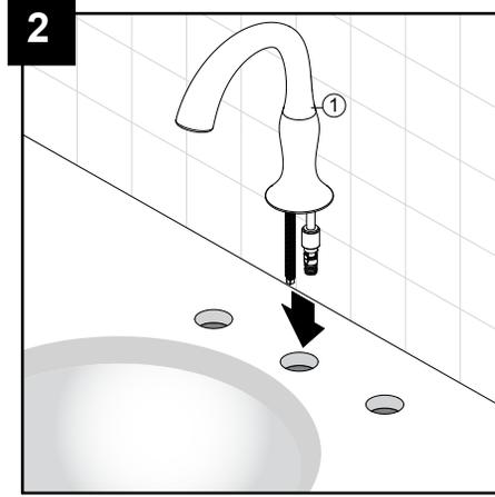
Place the spout assembly (1) through the mounting hole in sink.
