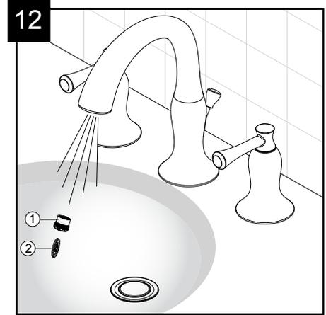
IMPORTANT: After installation is complete, remove the aerator (1) with a coin (2) to flush the water lines. Turn on the water supply and allow both hot and cold water to run for at least one minute each. This flushes away any debris that could cause damage to internal parts. While the water is running, check for leaks. Turn off the water and replace the aerator.
