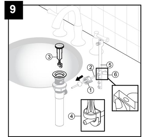
Remove the pivot nut (1). Install the horizontal rod (2) and the stopper (3), as shown (4). Hand tighten the pivot nut (1). Attach the horizontal rod (2) to the strap (5) using the clip (6).
