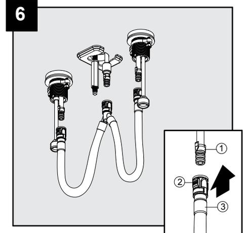
Align the tabs (1 & 2) on the quick connect assembly (3). Push the quick connect assembly (3) firmly upward and snap it onto the receiving tube tab. Pull down moderately to ensure the connection has been made. If it is necessary to remove the quick connect assembly (3), squeeze the tabs on the hose, and then pull down to disconnect.
