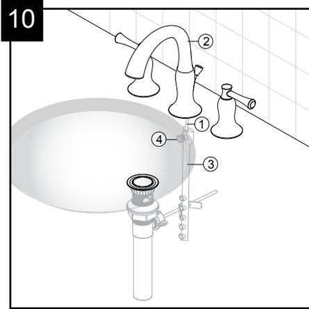
Insert the lift rod (1) through the spout assembly (2) and into the strap (3). Tighten the screw (4).
