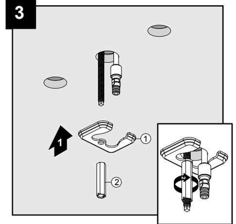
Secure the spout assembly with the washer (1) and nut (2).
