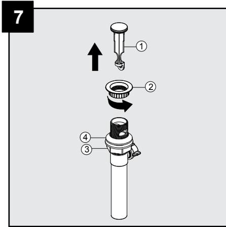
Remove the stopper (1) and the flange (2). Screw the nut (3) all the way down, and push the gasket (4) down.
