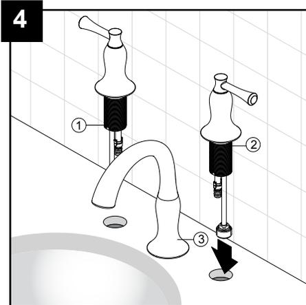
Slide the hot and cold end valves (1 & 2) through the sink mounting holes. Make sure the long tubes are installed away from the spout assembly (3). NOTE: The hot side end valve is labeled.
