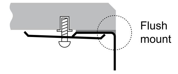
exposed approximately 1/4" from the edge of counter top opening. To achieve a reveal mount, leave the periforated line along the template.
