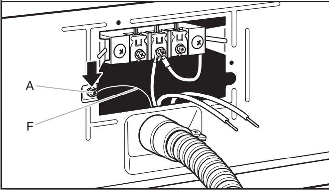
Connect ground wire (green or bare) (F) of direct wire cable under green external ground conductor screw (A). Tighten screw.
