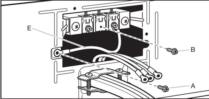
Install the correct strain relief for your electrical connection method, as shown on page 8 or 10.
