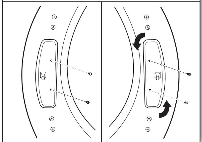
Using a TORX T25® screwdriver, remove the 2 screws securing the door strike to the door frame of the dryer. Rotate the strike 180° and attach to the opposite side of dryer door frame, as shown.
