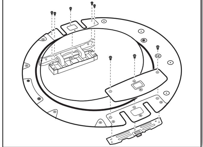
Using a TORX T25® screwdriver, reinstall the latch plate and latch backing plate with the 3 TORX® screws removed earlier and the hinge assembly with the 5 screws on the opposite sides from which they were removed.
