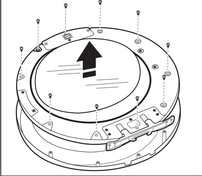
Position the door with the inside of the door facing up. Using a Phillips screwdriver, remove the 10 screws securing the inner door to the outer door. Lift off the inner door and set aside.
