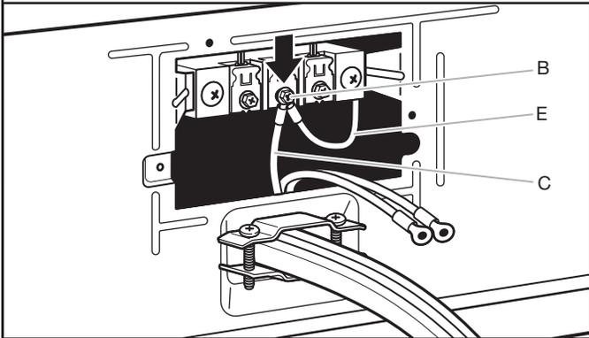
Connect neutral ground wire (E) and neutral wire (white or center wire) (C) of power supply cord or cable under center terminal block screw (B). Tighten screw.
