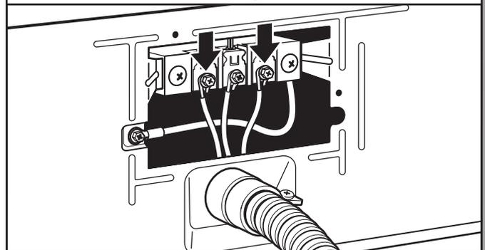
Place hooked ends of remaining direct wire cable wires under outer terminal block screws (hooks facing right). Squeeze hooked ends together and tighten screws. Finally, reinsert tab of terminal block cover into slot of dryer rear panel. Secure cover with hold-down screw. Now, go to "Venting Requirements."
