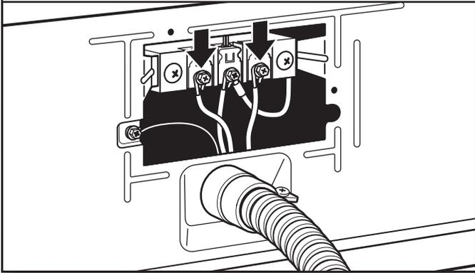
Place hooked ends of remaining direct wire cable wires under outer terminal block screws (hooks facing right). Squeeze hooked ends together and tighten screws. Finally, reinsert tab of terminal block cover into slot of dryer rear panel. Secure cover with hold-down screw. Now, go to "Venting Requirements."
