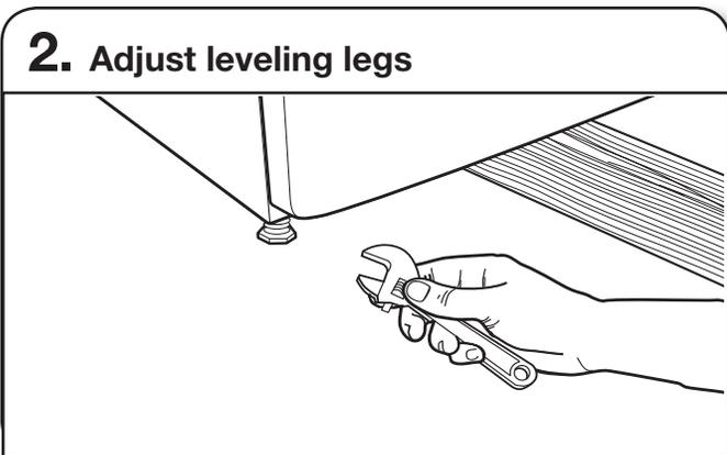
If dryer is not level, prop up using a wood block, use wrench to adjust legs up or down, and check again for levelness. Once dryer is level, make sure all four legs are snug against the floor and dryer does not rock.
