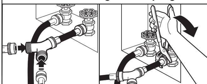
Attach one of the 5 ft (1.5 m) inlet hose ends to the "Y" connector. Attach washer cold inlet hose to other side of "Y" connector. Screw on coupling by hand until it is seated on connector. Using pliers, tighten the couplings an additional two-thirds turn.
