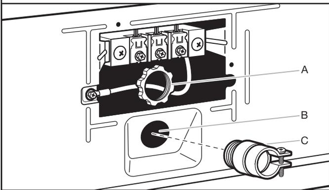
Unscrew the removable conduit connector (A) and any screws from a 3/4" (19 mm) UL listed strain relief (UL marking on strain relief). Put the threaded section of the strain relief (C) through the hole below the terminal block opening (B). Reaching inside the terminal block opening, screw the removable conduit connector (A) onto the strain relief threads and tighten securely.
