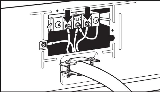
Connect remaining wires under outer terminal block screws. Tighten screws. Finally, reinsert tab of terminal block cover into slot of dryer rear panel. Secure cover with hold-down screw. Now, go to "Venting Requirements."
