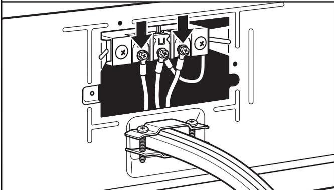
Place ends of remaining wires under outer terminal block screws. Tighten screws.
