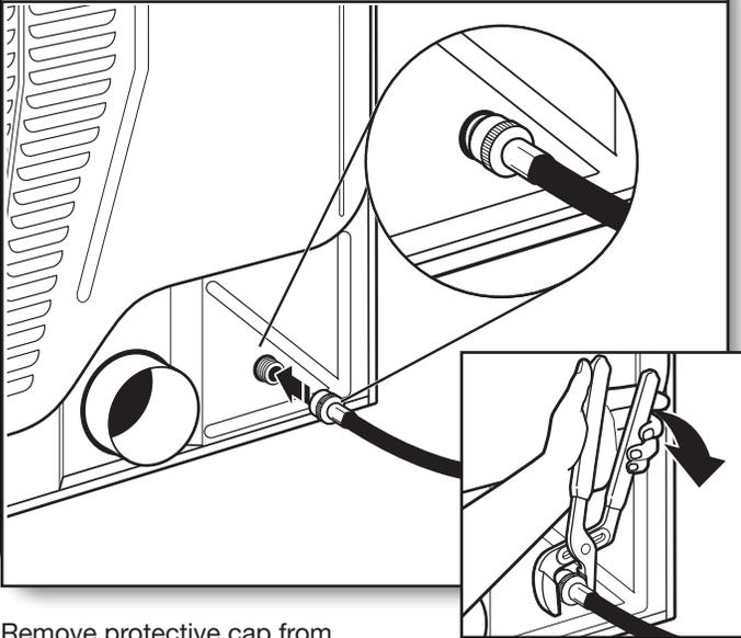
Remove protective cap from water inlet valve. Attach other end of long hose to fill valve at bottom of dryer back panel. Screw on coupling by hand until it is seated on fill valve connector. Using pliers, tighten the couplings an additional two-thirds turn.
