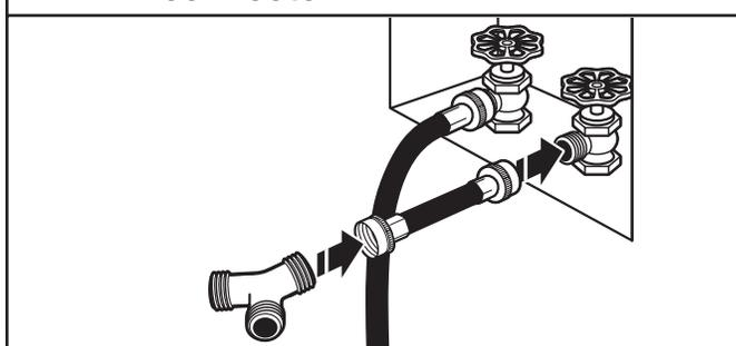
Attach 2 ft (0.6 m) inlet hose to cold water faucet. Screw on coupling by hand until it is seated on faucet. Then attach "Y" connector to male end of the 2 ft (0.6 m) inlet hose. Screw on coupling by hand until it is seated on connector.
