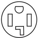
Power supply cord 4-wire receptacle (NEMA Type 14-30R):
