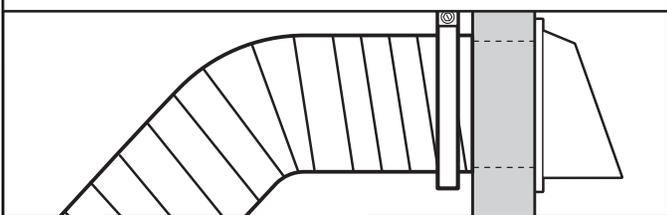
Vent must fit over the exhaust hood. Secure vent to exhaust hood with 4" (102 mm) clamp. Run vent to dryer location using straightest path possible. Avoid 90° turns. Use clamps to seal all joints. Do not use duct tape, screws, or other fastening devices that extend into interior of vent to secure vent, because they can catch lint.
