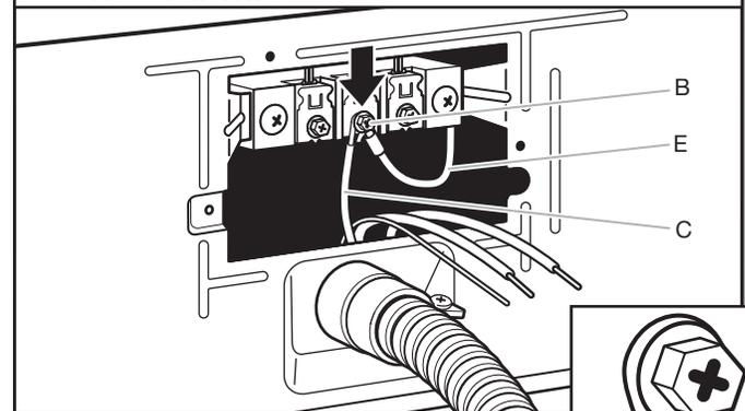
Connect neutral ground wire (E) and place hooked end (hook facing right) of neutral wire (white or center wire) (C) of direct wire cable under center screw of terminal block (B). Squeeze hooked ends together and tighten screw.
