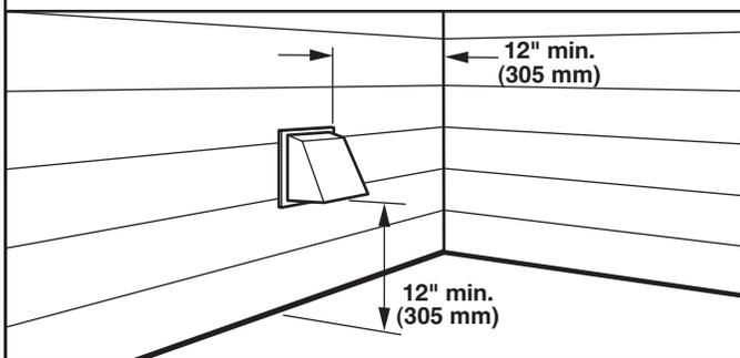
Install exhaust hood and use caulking compound to seal exterior wall opening around exhaust hood.
