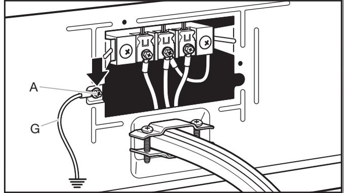
Connect a separate copper ground wire (G) under the green external ground conductor screw (A) to an adequate ground. Finally, reinsert tab of terminal block cover into slot of dryer rear panel. Secure cover with hold-down screw. Now, go to "Venting Requirements."
