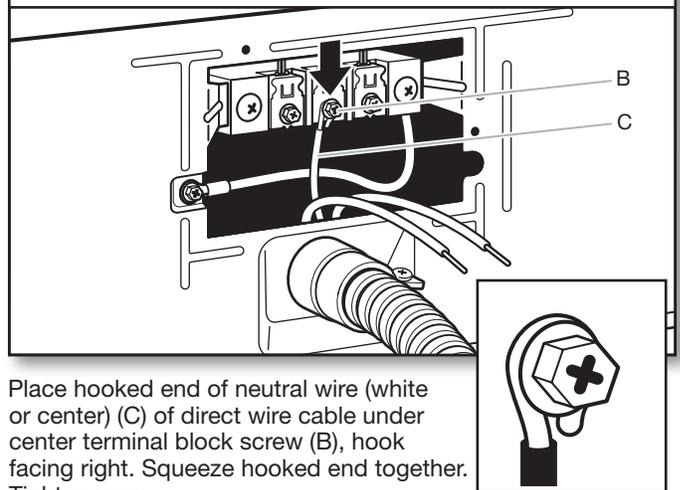
Place hooked end of neutral wire (white or center) (C) of direct wire cable under center terminal block screw (B), hook facing right. Squeeze hooked end together. Tighten screw.
