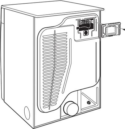
Remove hold-down screw and terminal block cover.
