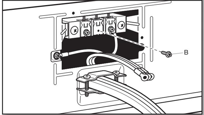
Remove center terminal block screw (B).
