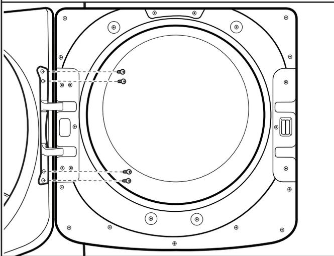
Using a TORX T25® screwdriver, remove the 4 screws securing the door hinge to the dryer and lift up and out to remove the door. Place the door on a soft towel or other non-scratch surface. Retain or set aside the 4 screws.
