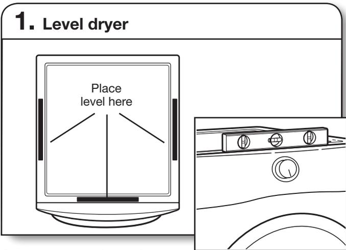
Check levelness of dryer from side to side. Repeat from front to back.
