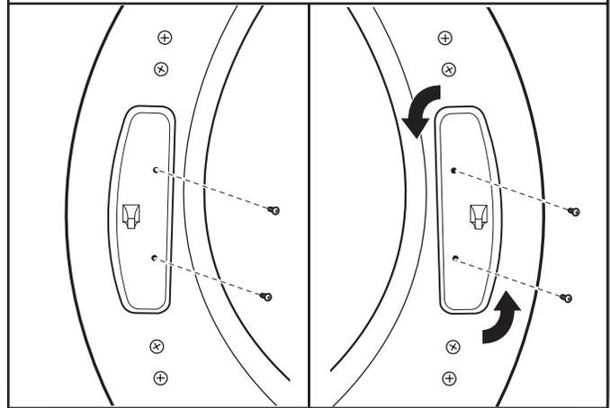
Using a TORX T25<sup>®</sup> screwdriver, remove the 2 screws securing the door strike to the door frame of the dryer. Rotate the strike 180° and attach to the opposite side of dryer door frame, as shown.
