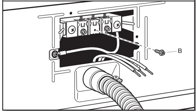
Remove center terminal block screw (B).
