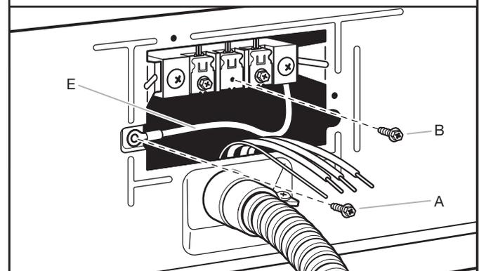
Remove center terminal block screw (B). Remove neutral ground wire (E) from green external ground conductor screw (A).
