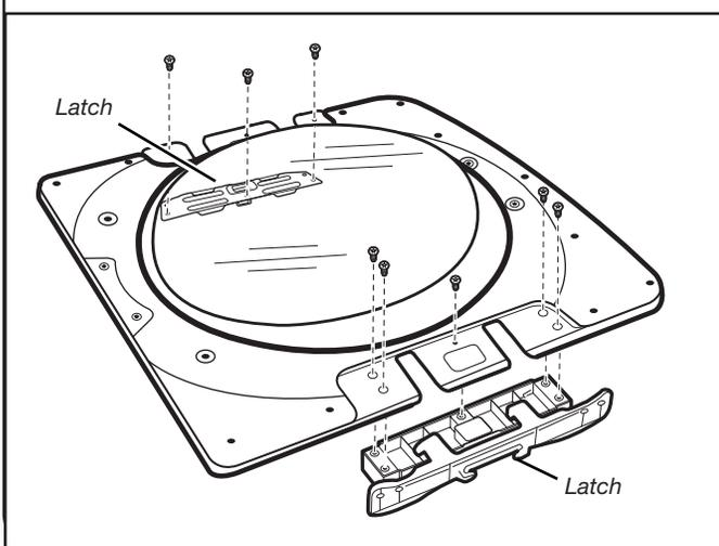
Using a TORX T25® screwdriver, reinstall the latch plate and hinge assembly on the opposite sides from which they were removed.
