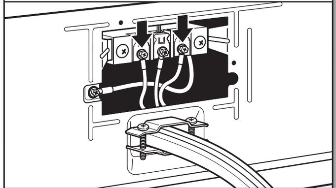
Connect remaining wires under outer terminal block screws. Tighten screws. Finally, reinsert tab of terminal block cover into slot of dryer rear panel. Secure cover with hold-down screw. Now, go to "Venting Requirements."
