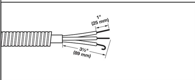
Direct wire cable must have 5 ft. (1.52 m) of extra length so dryer may be moved if needed.
