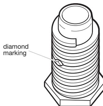
Examine leveling legs, find diamond marking. Screw legs into leg holes by hand – use a wrench to finish turning legs until diamond marking is no longer visible.
