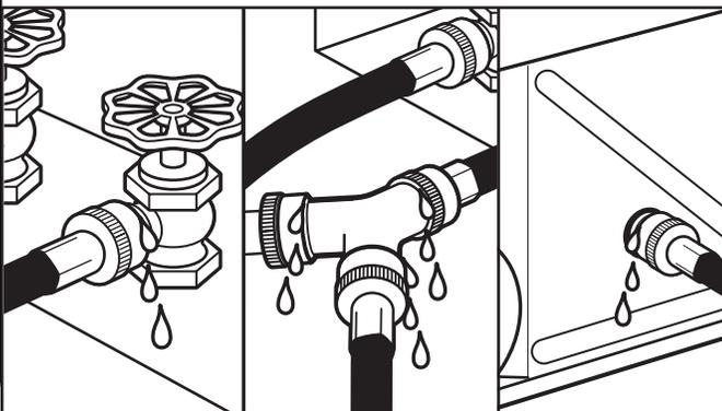
Check for leaks around "Y" connector, faucet, and hoses.
