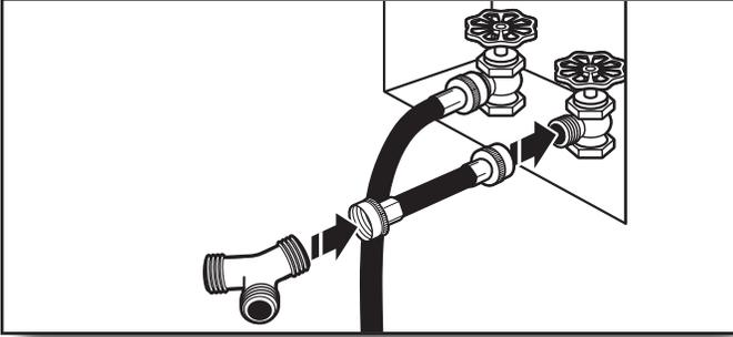
Attach 2 ft (0.6 m) inlet hose to cold water faucet. Screw on coupling by hand until it is seated on faucet. Then attach "Y" connector to male end of the 2 ft (0.6 m) inlet hose. Screw on coupling by hand until it is seated on connector.
