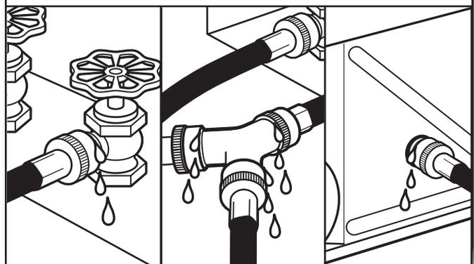
Check for leaks around "Y" connector, faucet, and hoses.
