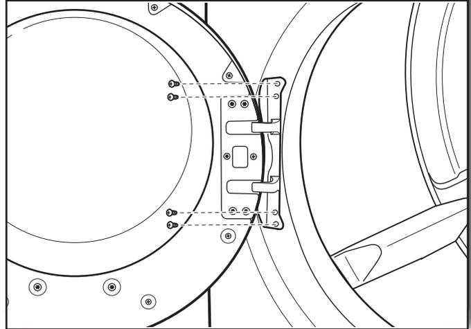
Using a TORX T25® screwdriver, remove the 4 screws on the dryer. Insert the tabs on the hinge into the mounting slot and slide down to engage the top tab. Secure in place with the 4 TORX T25® screws removed earlier.
