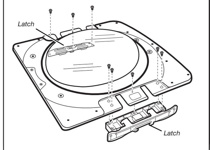
Using a TORX T25® screwdriver, reinstall the latch plate and hinge assembly on the opposite sides from which they were removed.
