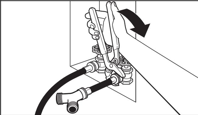
Using pliers, tighten the couplings with additional two-thirds turn.
