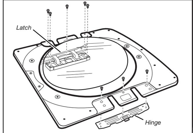
Using a TORX T25® screwdriver, remove the 3 TORX® screws securing the latch plate and the 5 screws holding the hinge assembly in place.
