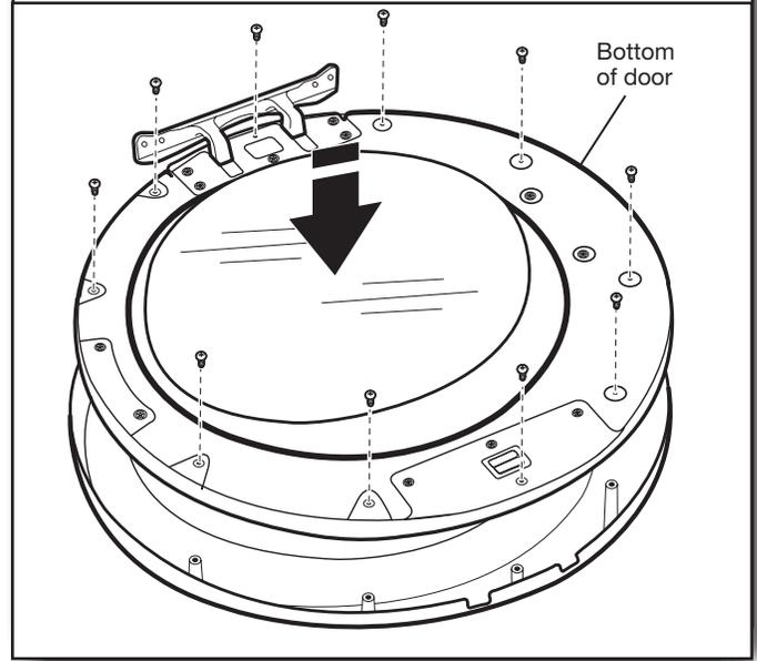
Position the door with the inside of the door facing up. Reinstall the 10 screws securing the inner door to the outer door.
