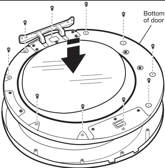
Position the door with the inside of the door facing up. Reinstall the 10 screws securing the inner door to the outer door.
