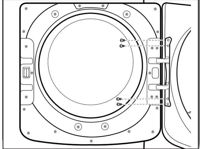
Using a TORX T25® screwdriver, reinstall the 4 screws securing the door hinge to the dryer.
