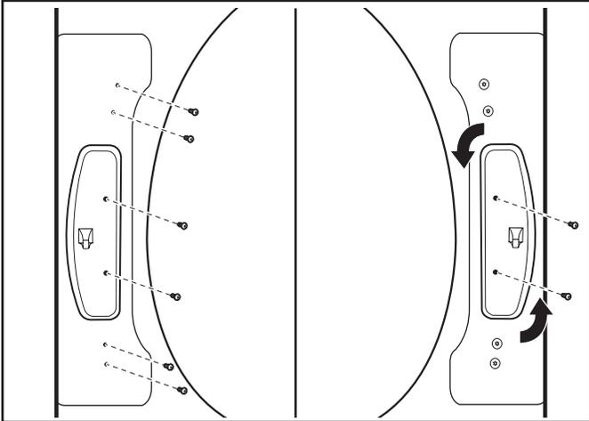
Using a TORX T25® screwdriver, remove the 2 screws securing the door strike to the door frame of the dryer. Remove the 4 screws above and below the door strike and set aside for later use. Rotate the strike 180° and attach to the opposite side of dryer door frame, as shown.
