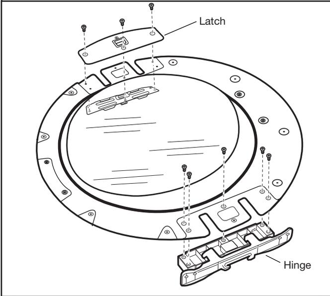
Using a TORX T25® screwdriver, remove the 3 TORX® screws securing the latch plate and latch backing plate and the 5 screws holding the hinge assembly in place.
