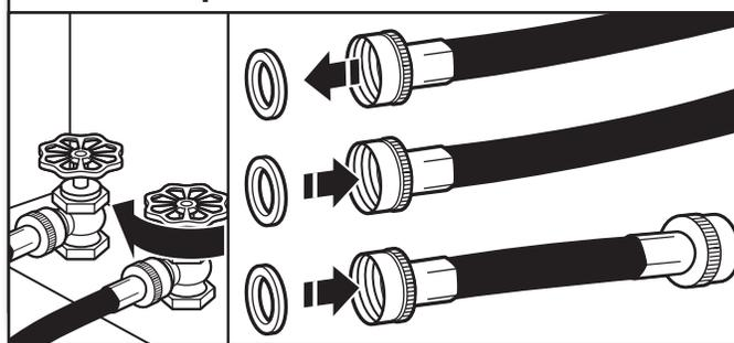
Turn cold water faucet off and remove washer inlet hose.
