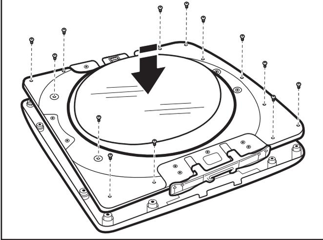
Position the inner door on the outer door assembly. Using a Phillips screwdriver, secure with the 13 screws removed earlier.
