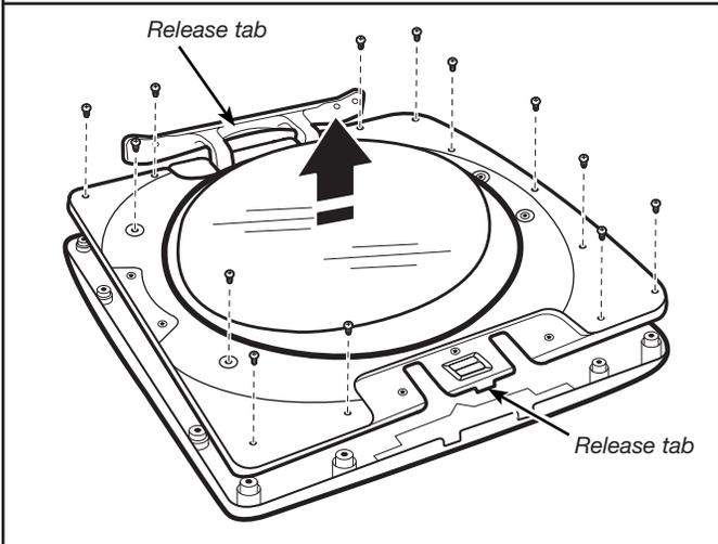
Position the door with the inside of the door facing up. Using a Phillips screwdriver, remove the 13 screws securing the inner door to the outer door. Lift off the inner door and set aside.
