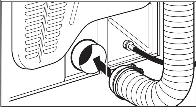
Using a 4" (102 mm) clamp, connect vent to exhaust outlet in dryer. If connecting to existing vent, make sure vent is clean. Dryer vent must fit over dryer exhaust outlet and inside exhaust hood. Check that vent is secured to exhaust hood with a 4" (102 mm) clamp.
