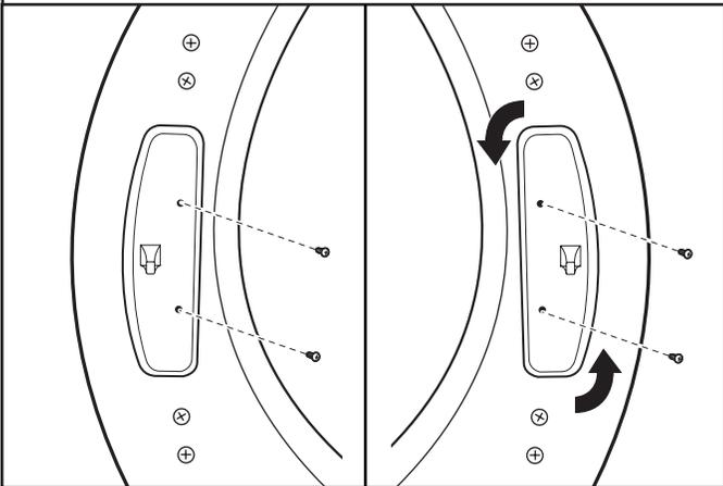
Using a TORX T25® screwdriver, remove the 2 screws securing the door strike to the door frame of the dryer. Rotate the strike 180° and attach to the opposite side of dryer door frame, as shown.
