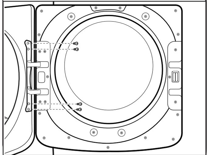
Using a TORX T25® screwdriver, remove the 4 screws securing the door hinge to the dryer and lift up and out to remove the door. Place the door on a soft towel or other non-scratch surface. Retain or set aside the 4 screws.
