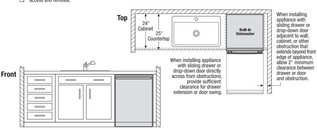
Use these dimensions and clearance instructions for planning purposes only. For detailed installation instructions, refer to installation guide, packed with product, or on the web at frigidaire.com.
