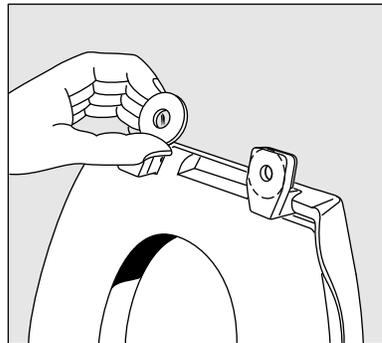
Attach washer to bottom of hinge. Remove paper backing.
