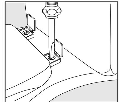
Use a screwdriver to tighten bolt.
