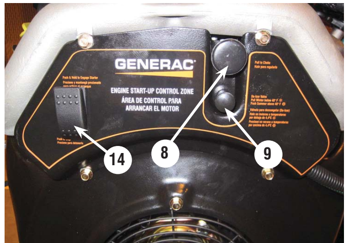
Figure 6 - Engine Control Panel
