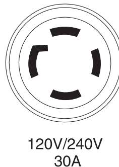
Figure 12 - 120/240 VAC, 30 Amp Receptacle
