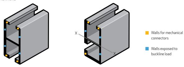
Thickness of walls for mechanical connections: min. 0.156 inch (4.0mm) Thickness of walls exposed to buckling load: min. 0.08 inch (2.0mm) Moment of Inertia for profile area about X-X: min. 0.4 inch<sup>4</sup> (19.2cm<sup>4</sup>)
