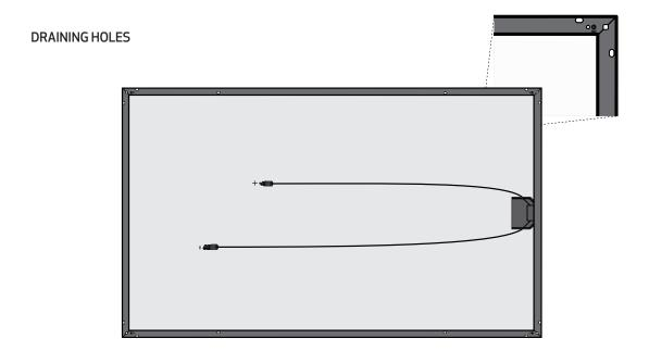
The maximum load the module should be subjected to must not exceed the module design load of  $75.2 \, \text{lb/ft}^2$  (3600 Pa) (UL1703) respectively maximum module load of  $551 \, \text{kg/m}^2$  (5400 Pa) (IEC61215). Site-specific loads such as wind and snow need to be taken into consideration to ensure that this weight loading is not exceeded.
