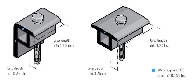
Use clamps of extruded aluminum with minimum yield strength of 2089 ton /  $ft^2$  (200 MPa) and minimum tensile strength of 2610 ton /  $ft^2$  (250 MPa), i.e. 6005 T5 alloy, with a minimum grip length of 1.75 inches (44.5 mm), minimum grip depth of 0.2 inches (5 mm) and a minimum thickness of load carrying walls of 0.16 inches (4 mm). Use size 5/16″ stainless steel bolted connections with 5/16″ split washer. The applied torque to fasten the clamps must be within the range of 9 ft lbs (12 Nm).
