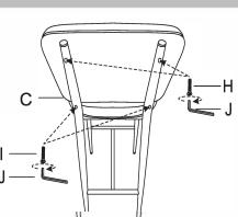
STEP 5B: Attach Seat Back (Part C) to the upper part of the Metal Tube Frame (Part A) using M6\*35 Screws (Part H) and Large Allen Wrench (Part J)
