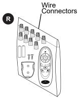
Connect all GROUND (GREEN) wires from fan (on downrod (A), if applicable, mounting bracket (C)) and remote control receiver (Q) to BARE/GREEN supply wire from ceiling.
