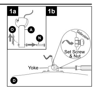
Insert downrod (A) through canopy (B) and yoke cover (E). Thread wires from motor housing (D) up through downrod (A).
