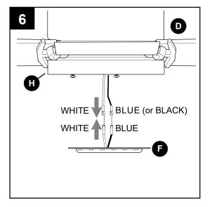
Carefully arrange wiring within the fitter plate (H) to ensure wires do not get pinched when attaching the LED light kit (F).
