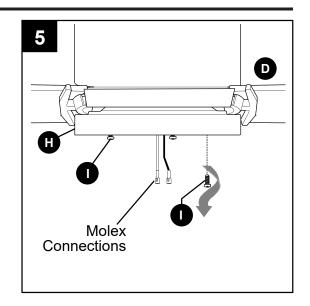
Connect WHITE wire from LED light kit (F) to WHITE wire from motor housing (D). Connect BLUE wire from LED light kit (F) to BLUE (or BLACK) wire from motor housing (D). Make sure molex connections are secure.
