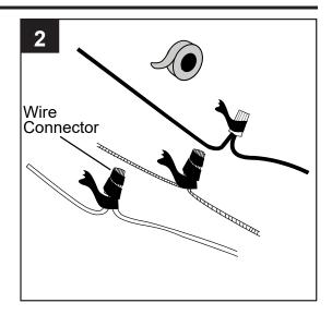
Gently slide remote control receiver (Q) flat-side up into mounting bracket (C). Turn spliced/taped wires upward and gently push wires and wire connectors (CC) into outlet box. Let antenna from remote control receiver (Q) hang to the side.
