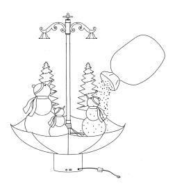
Turn off the switch. Evenly distribute the snowflakes into the umbrella shaped base. It is suggested to keep an appropriate amount of snowflakes aside, for when some fall out.
