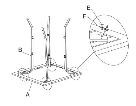
Connect Leg Connector (Part C) with Legs (Part B) using screws (E) and Washer (F) as shown in diagram.
